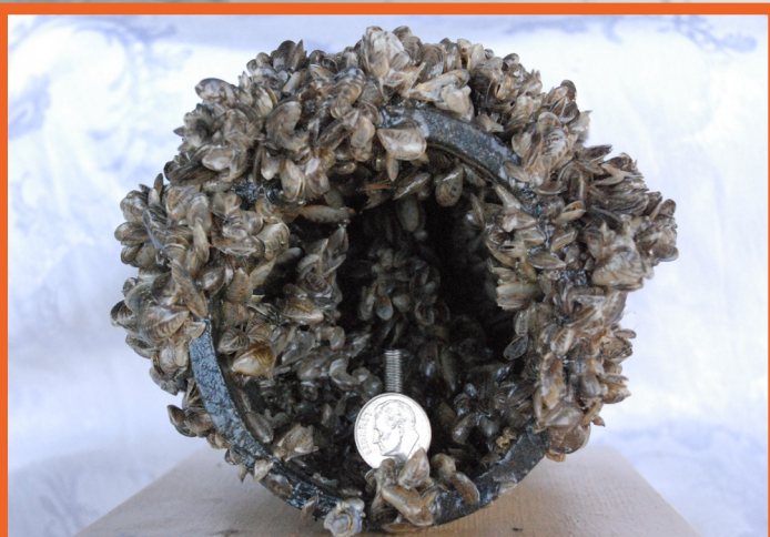
This pipe has been so infested with zebra mussels that water would have a difficult time passing through it.
